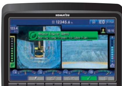
Eco-gauge, Eco guidance and fuel consumption gauge
