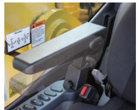
Armrest with simple height adjustment
