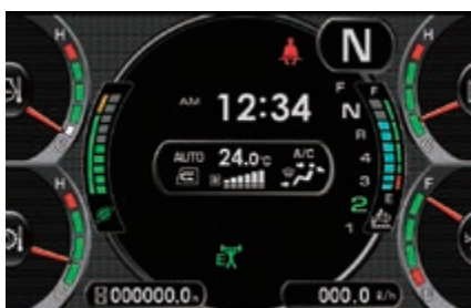
Information at a glance: basic dashboard LCD monitor
