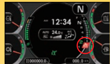
AdBlue® level gauge and refill guidance
