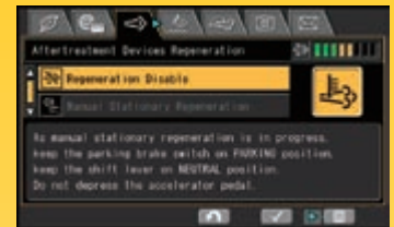
Aftertreatment device regeneration screen for the KDPF
