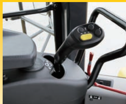
Advanced joystick steering system
