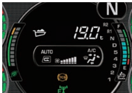
Payload meter displays the loaded weight
