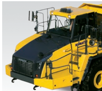
Built-in ROPS/FOPS to ISO 3471 and SAE J1040-1988c standards
